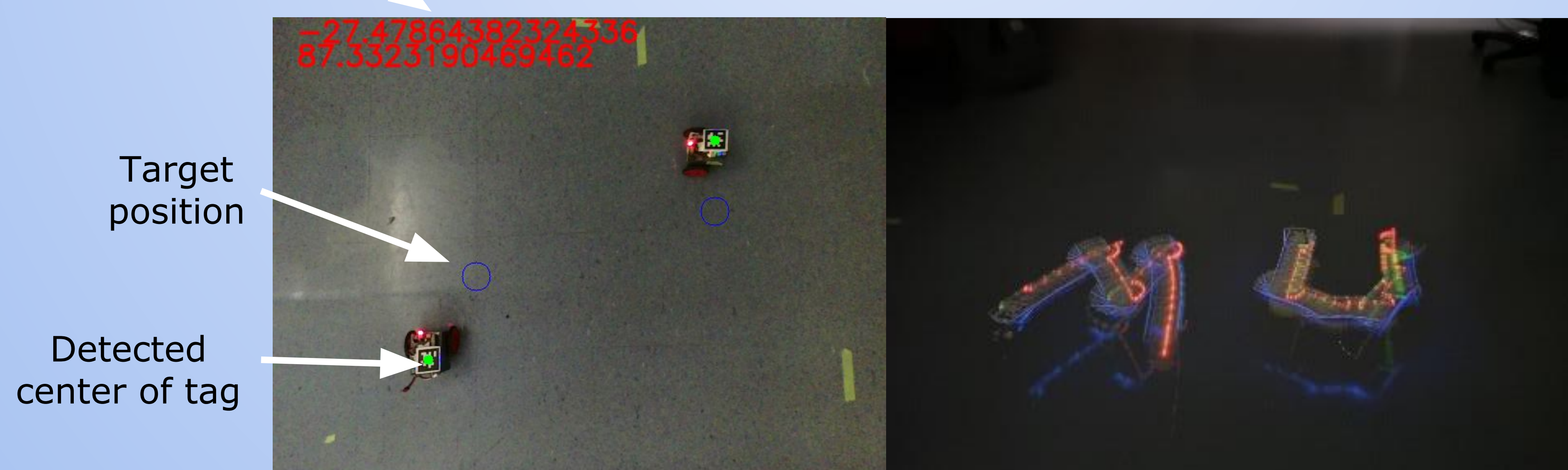
(Left) Camera's view with information overlaid. (Right) long-exposure photo of agents moving on their path.
