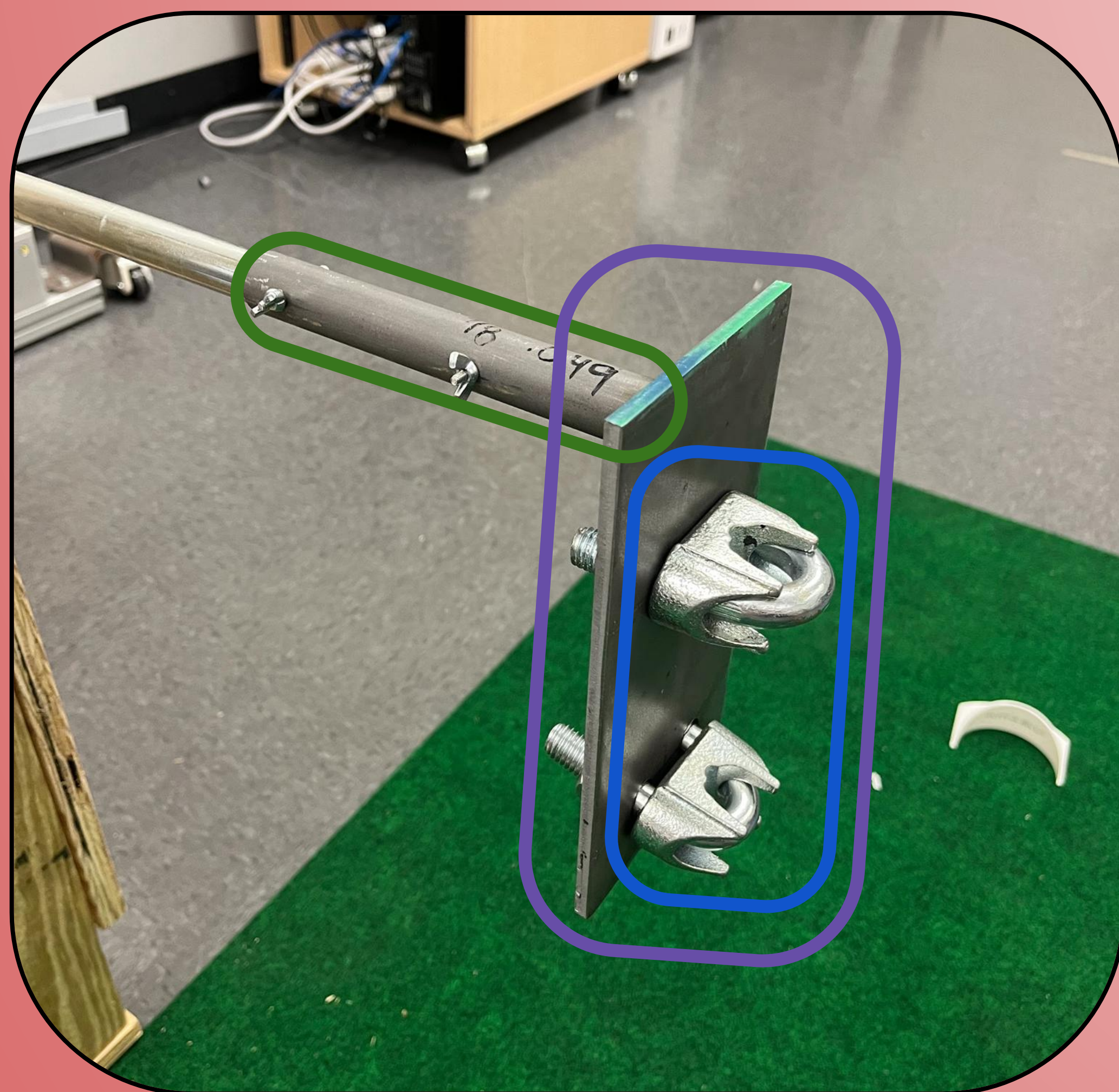
Metal pipe welded to a steel plate with U-bolts to hold the putter in place
